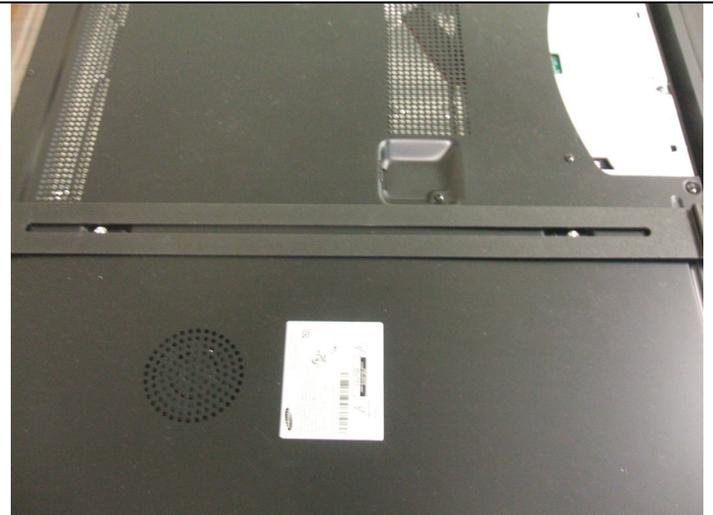
**Step 8** – Place the wall hanging bracket (Supplied by you) on top of the speaker bracket and install the mounting screws but **DO NOT TIGHTEN THE SCREWS** – the bracket needs to be able to move freely.
