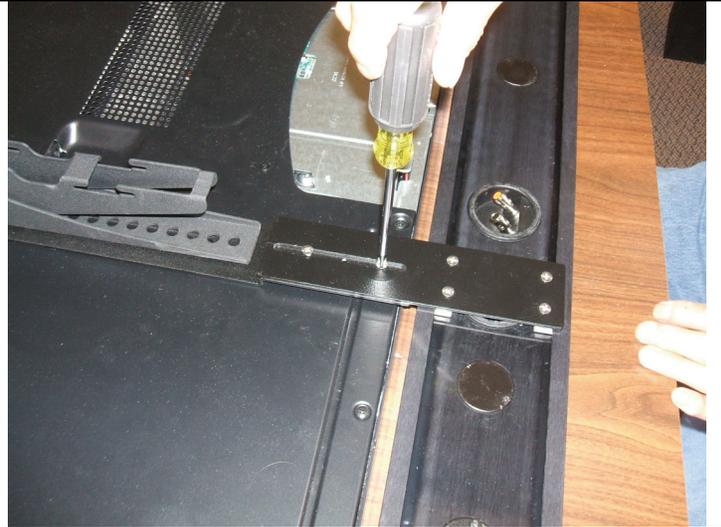
**Step 14** – Tighten the screws that hold the brackets and TV mount to the rear of the TV and that the speaker is tight against the bottom of the TV – we want to minimize any gaps here for the best esthetic.
