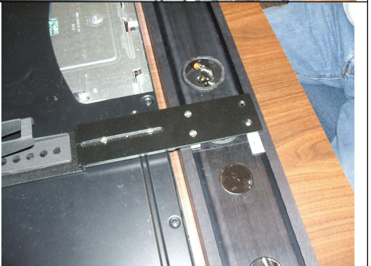
**Step 13** – At this point, both brackets are loose and can be moved up and down and the speaker can slide left and right.
