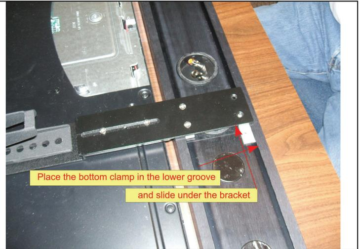
**Step 11** – Slide the bottom clamp fully under the bracket while aligning the 2 screw holes in the bracket with the 2 screw holes in the lower clamp.
