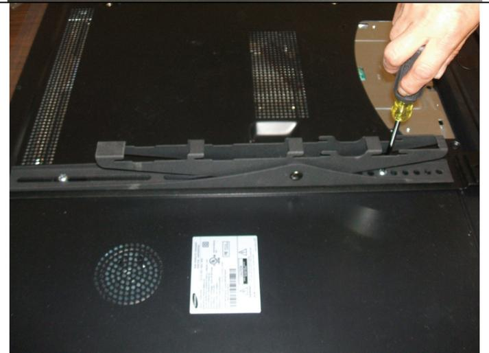
**Step 9** – Since all the screws are loose, you can slide the upper clamp into the upper groove in the rear of the speaker.
